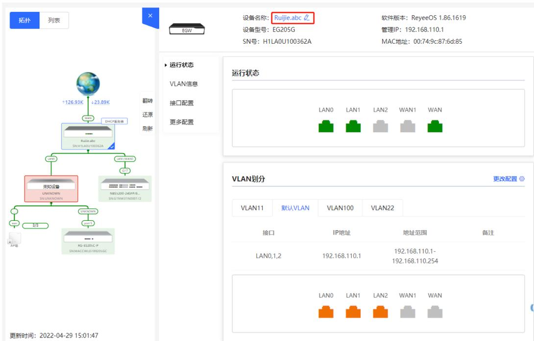
The screenshot shows the network management interface. On the left is a network topology diagram with a central router (Ruijie\_20G) connected to other devices. On the right is the configuration panel for the selected device 'Ruijie.abc'. The panel includes:
