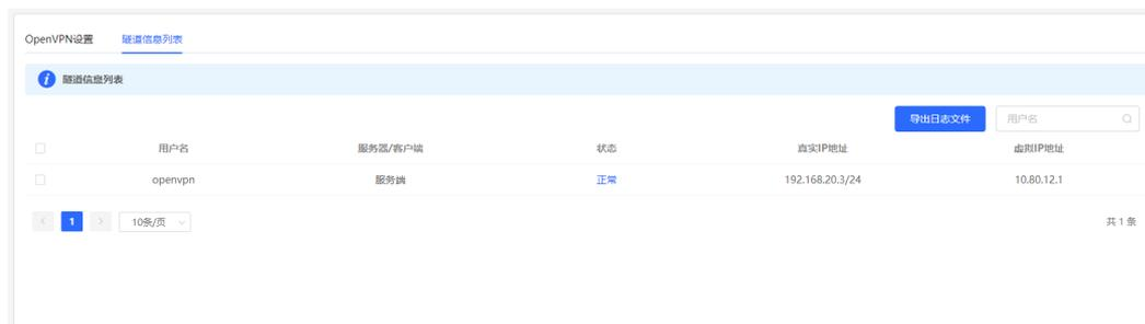
The screenshot shows the 'OpenVPN设置' (OpenVPN Settings) page with the '隧道信息列表' (Tunnel Information List) tab selected. It displays a table with columns for '用户名' (Username), '服务器/客户端' (Server/Client), '状态' (Status), '真实IP地址' (Real IP Address), and '虚拟IP地址' (Virtual IP Address). A '导出日志文件' (Export Log File) button and a search box are also visible.
